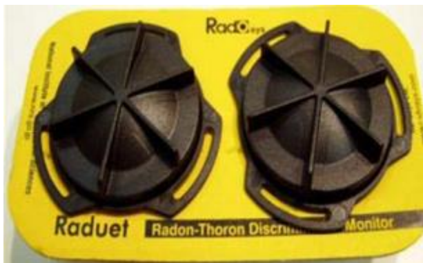
Figure 2. Raduet nuclear track detector produced in Radosys, Hungary
