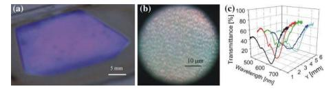
**Fig. 3** a Image of the DCP sample, the scale bar is 5 mm; **b** zoomed part of the image **a** obtained using  $\times$ 40 objectives, and microscopic set-up shown in Fig. 1c. The scale bar is 10 µm; **c** transmission spectra obtained from different areas (each of diameter of 50 µm) of the DCP sample, with 1 mm distance between two adjacent areas
