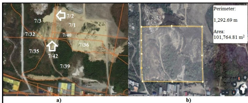
Figure 10 Maps: a) Location of cadastre plots (National Spatial Data Infrastructure, 2019) and b) the real area of the surveyed terrain (Google Earth)
