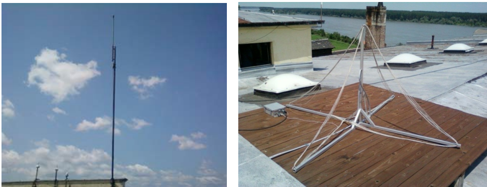
Belgrade VLF receiver stations: AbsPal (left) and AWESOME (right) antennas.
