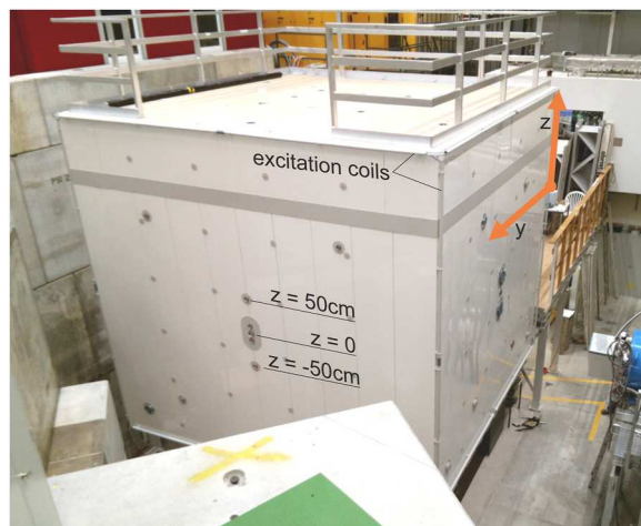
FIG. 5. View of the rear side of the MSR. Two of the tubes carrying the excitation coils used to measure the shielding factor are indicated. The openings used for the horizontal scans along the y axis (see Fig. 14) are labeled with their z-coordinates.
