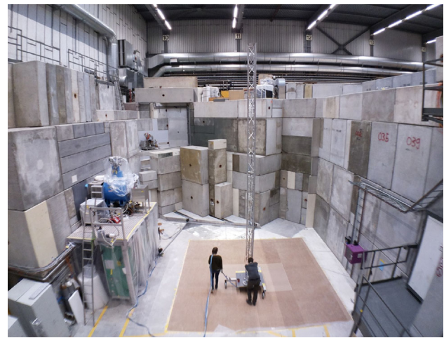
Fig. 2 Picture taken during a magnetic-field mapping in UCN area South at PSI [18]. The area was emptied before the n2EDM experiment was set up. Two people are moving the ‘mapping tower’ around. About half height of the tower in the displayed position marks the center of n2EDM. The UCN source is behind the concrete shielding to the left, and a superconducting magnet (blue) to fully polarize UCN directed to n2EDM, is visible on the platform. See main text for further details
