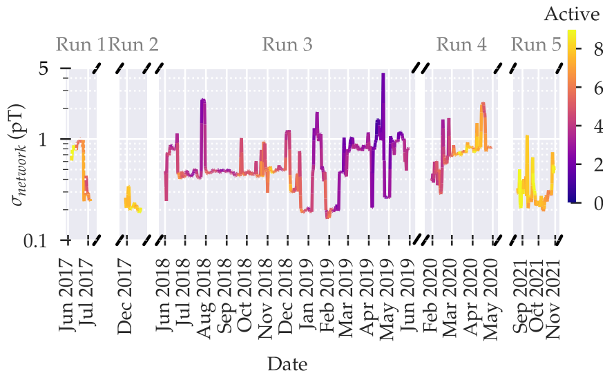
FIG. 2. One-day rolling average of the GNOME noise level according to Eq. (10) over the course of the first five Science Runs. The standard deviation at each magnetometer is calculated using the data for one second. Then this information is averaged for one hour. The color of the line indicates the number of active stations as indicated on the color map legend at the upper right.
