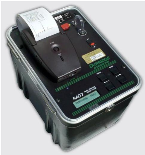
Figure 2. Radon continual monitor, Rad7- Durridge Co, USA
