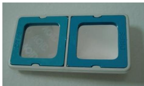
Figure 2a. Direct Radon Progeny Sensor
