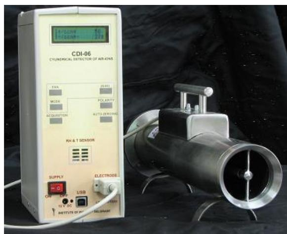
Figure 1. Cylindrical Detector of Air-Ions (CDI-06)
