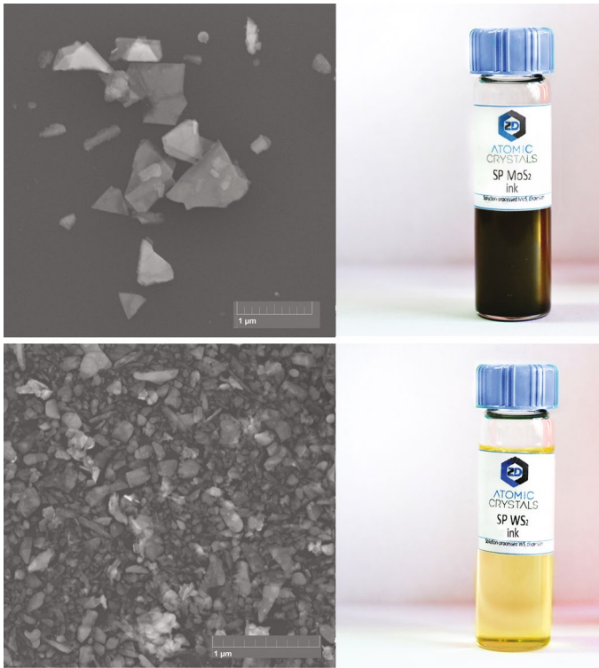
Fig. 3 MoS 2 (up) and WS 2 (down) flakes on Si/SiO 2 substrate—Tescan MIRA3 field-emission gun SEM-left. Photos of MoS 2 and WS 2 dispersions-right
