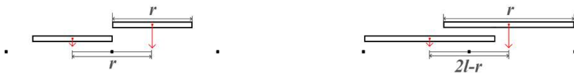
Figure 3.6: Illustration of equivalency of two models: (I) deposition of segments on localized adsorbing sites and (II) deposition of particles on extended lattice sites. On the left is a case of r < l and on the right a case of l < r < 2l .
