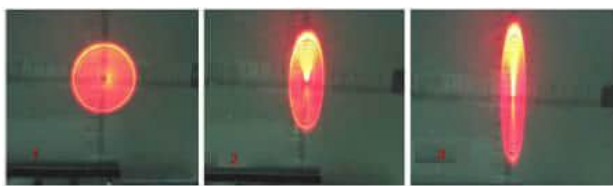
Figure 8 – Diffraction picture recorded after the TESHG microlens was: 1) formed; 2) and 3) stretched in one direction. Millimeter scale is visible.
