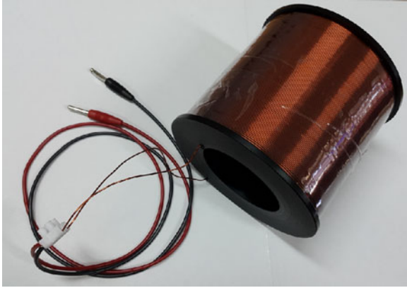
Fig. 11. Prototype of modified solenoid. The dimensions of modified solenoid prototype are R_{in} = 6 cm, L = 12.2 cm, D = 0.66 cm, l = 1.76 cm, d = 1.1 cm. It is wound using a 1-mm-diameter copper wire (1.1 mm with coating), and it has 979 turns. Its resistance, inductivity, and mass are measured to be 9 \Omega , 68.37 mH, and 3.6 kg, respectively. The spool thickness is 5 mm.
