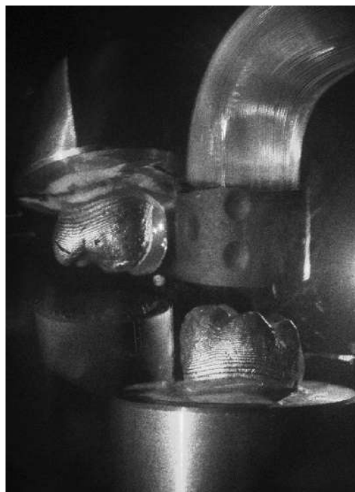
FIGURE 5.—The final interference pattern observed on a tooth model, after 120 s of polymerization. As in previous figure, a tooth model is on the right bottom part of a photograph, while its image is on the upper left. Polymerization LED light source is on the upper right corner, while its image is on the lower left.
