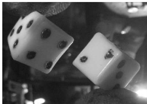
FIGURE 3.—An object (a dice on the right side) and its image in a spherical mirror (on the left). Observe that both front and back side of the same object are seen.
