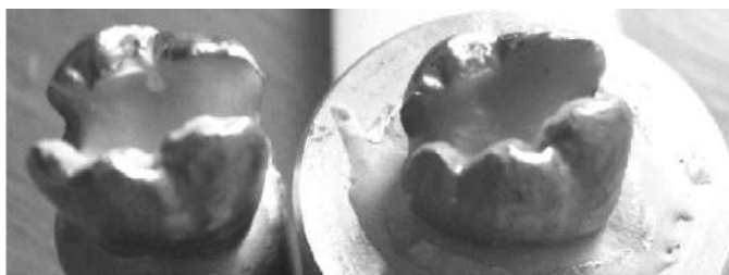
FIGURE 1.—Human molar with MOD cavity (left) and its mechanical model made of dental composite (right). They are both painted with silver paint, as required in holography.
