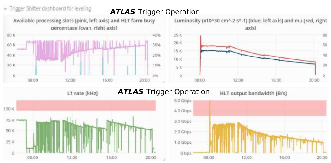
Figure 18. An example of a P-BEAST dashboard as used by the shifters during 2017 operation. The HLT farm availability (top left), the luminosity and the pile-up, 'mu' (top right), the total L1 accept rate (bottom left), and the total HLT output bandwidth (bottom right) are shown.
