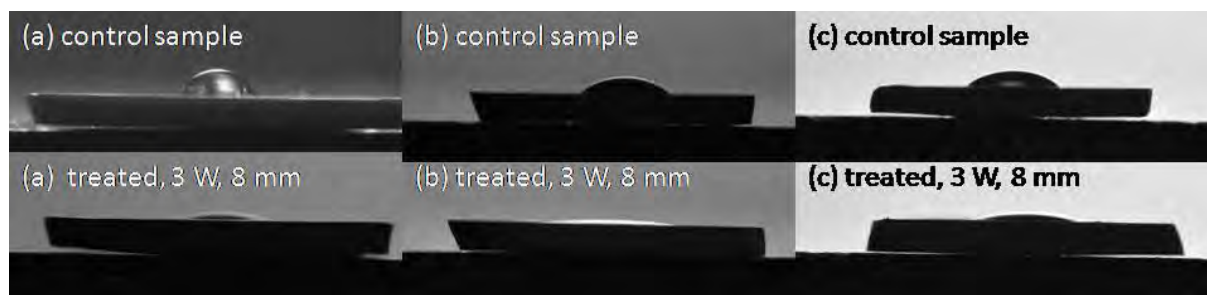
Fig. 1: Images for the contact angle for the three reference liquids: (a) distilled water, (b) ethylene glycol and (c) diiodomethane
