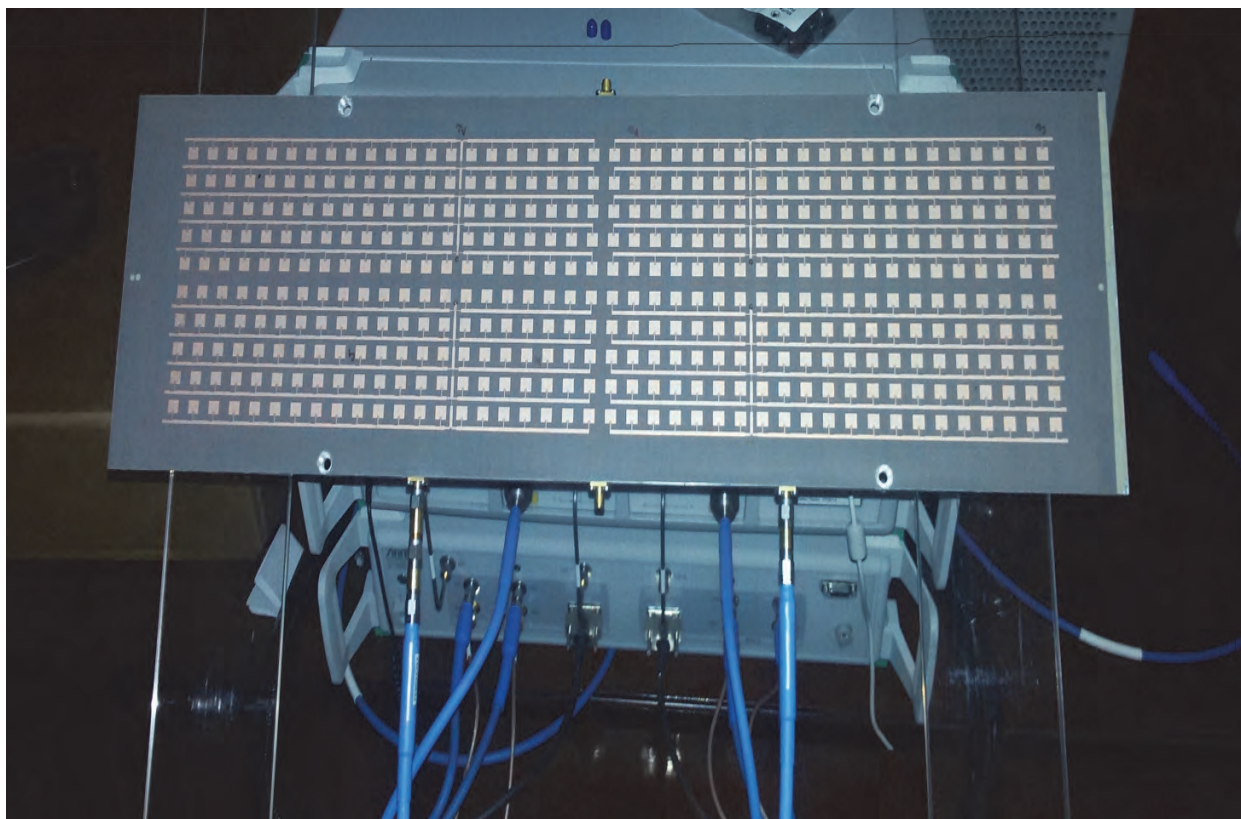
Fig. 6. Photograph of the manufactured patch antenna array. The antenna footprint is 31 \lambda_0 \times 7.5 \lambda_0
