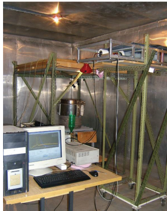
FIGURE 2. Detectors in the underground laboratory. Large scintillator detector is placed above HPGe and small scintillator can change position.
