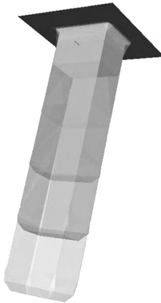
Figure 2. The time evolution of the profile during ion-enhanced chemical etching.
