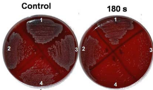
Fig. 4. Planktonic samples of S. aureus treated by plasma and afterwards cultivated on growth medium. Flow of He was 1 slm and the power was 1.6 W. Four different initial concentrations of bacteria were used: (1) 12 \cdot 10^8 CFU/ml; (2) 12 \cdot 10^7 CFU/ml; (3) 12 \cdot 10^6 CFU/ml; (4) 12 \cdot 10^5 CFU/ml.
