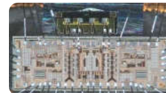
Figure 2: 64Gb/s PAM-4 transimpedance amplifier array
