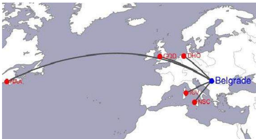
Figure 1. Great Circle Paths (GCPs) of subionospherically propagating VLF radio signals recorded at Belgrade site.
