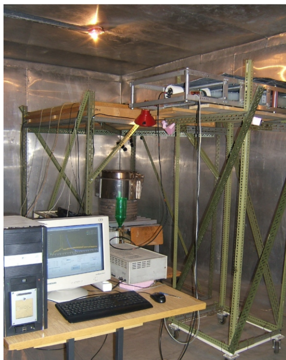
Figure 2. Detectors in the underground laboratory (UL). The big plastic scintillator is positioned over the HPGe detector, seen in its lead shielding. The small plastic scintillator is in the front upper right corner. A hermetically sealed, 1 mm Al lining covering the entire UL, which enables the doubly filtrated ventilation system to sustain an overpressure of 2 mbar and keeps the radon concentration at an average level of some 10 Bq/m 3 , is also shown
