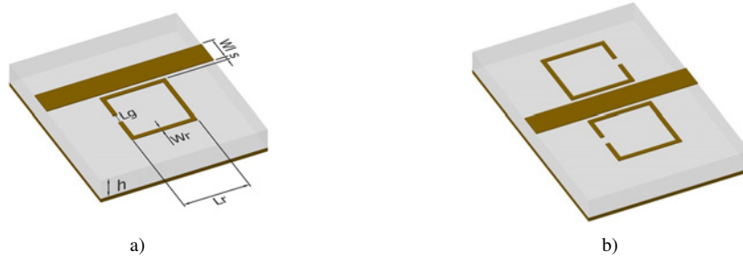
Fig. 1: Microstrip line coupled with a) one SRR with the gap in a perpendicular arm; b) two such SRRs placed anti-symmetrically. Dimensions: L_r = 3 mm, L_g = 0.5 mm, W_r = 0.2 mm, W_l = 1.2 mm, s = 0.1 mm.
