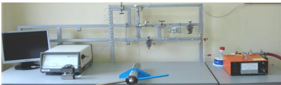
Figure 2. Apparatus for high pressure density measurements
