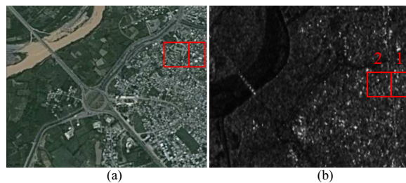
Figure 7. a)optical image of Kosar hospital in AstaneAshrafiye. b) Red box 1 is place of creating of fake targets, and red box 2 is place of creating of camouflage
