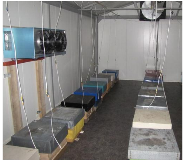
Fig.2. Developed bee hive temperature measurement system in real circumstances
