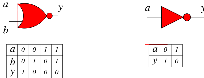
Figure 1.2. Universal set of classical logic gates. One universal set of classical logic gates consists of a NOR and a NOT gate. In this figure, these gates are represented by truth tables and a symbol in classical circuit model.
