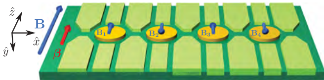
FIG. 1. (Color online) Parallel geometry: four quantum dots (yellow discs) aligned along the x axis in the presence of an external magnetic field \mathbf{B} that is applied parallel to the SOI vector \boldsymbol{\beta} (red arrow), which must be perpendicular to the line of the dots and which we take to be the z direction. At each dot, there is a local magnetic field \mathbf{B}_i (blue arrows), also assumed to be parallel to \mathbf{B} , but with alternating orientations as indicated. The direction of \mathbf{B} defines the spin quantization axis. The dots are defined electrostatically by metallic gates (light green structures). Each dot contains a spin-1/2, and the exchange ( J_{ij} ) and the SOI-induced ( \boldsymbol{\beta}_{ij} ) interactions between the spins can be controlled by changing the electrostatic potential between the dots. The dots 1 and 2 (from left to right) define the first ST qubit, and the dots 3 and 4 the second ST qubit.
