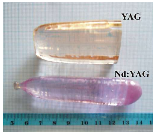
Fig. 2. A view of an obtained: (a) YAG and (b) Nd:YAG single crystals plate.
