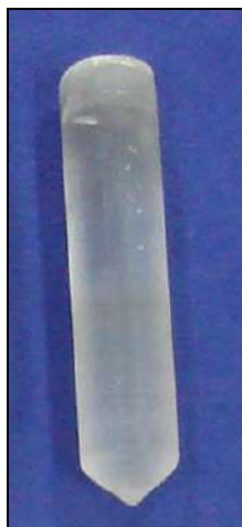
Fig. 2. Photographs of Bridgman-grown \text{CaF}_2 single crystal.
