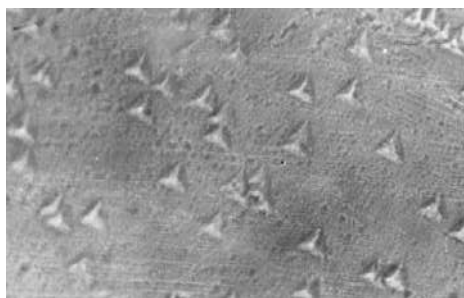
Fig. 3. The microscopic image of the surface \text{CaF}_2 crystal plate in the direction \langle 111 \rangle . Magnification of 270x
