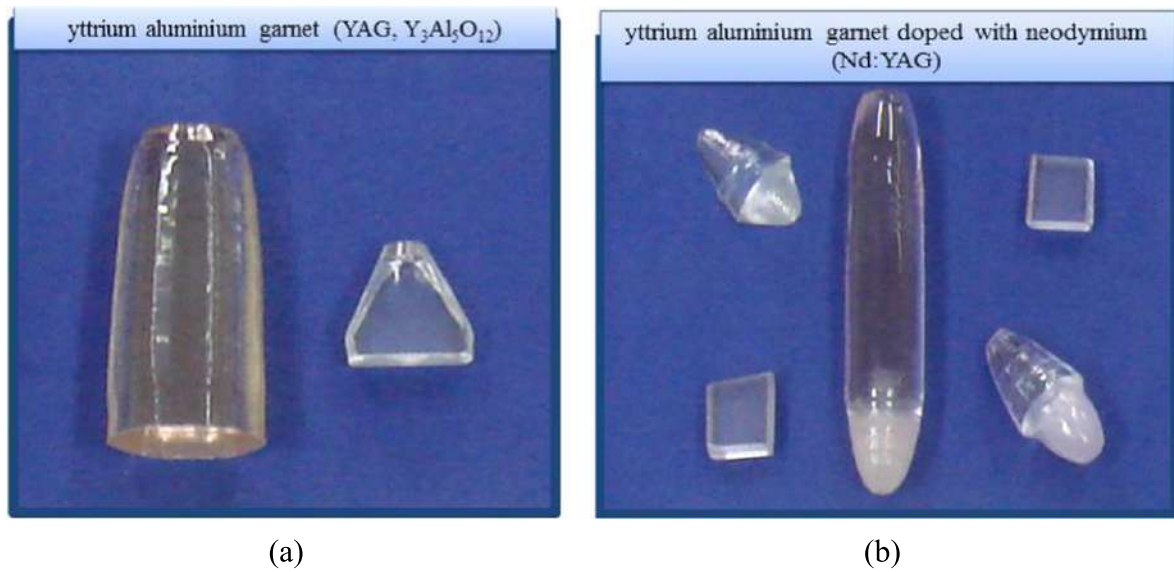
Figure 1 A view of an obtained (a) YAG and (b) Nd:YAG single crystals plate.
