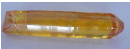
Fig. 5. Photographic image of the studied obtained crystal of Bi 12 GeO 20 .
