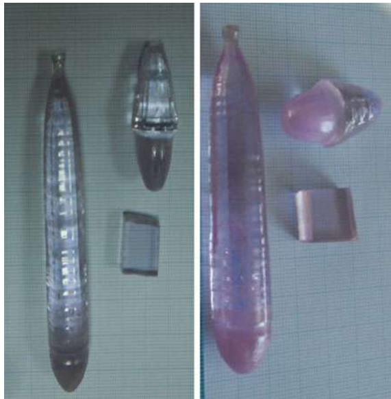
Fig. 2 A view of an obtained YAG ( \text{Y}_3\text{Al}_5\text{O}_{12} ) and Nd:YAG ( \text{Nd}:\text{Y}_3\text{Al}_5\text{O}_{12} ) single crystal plate
