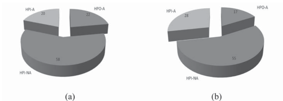
Figure 1. Characterization of DOM from the Danube: (a) before and (b) after ozonation
