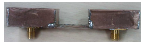
Fig. 10. Side view of fabricated ENZ waveguide with coaxial connectors.
